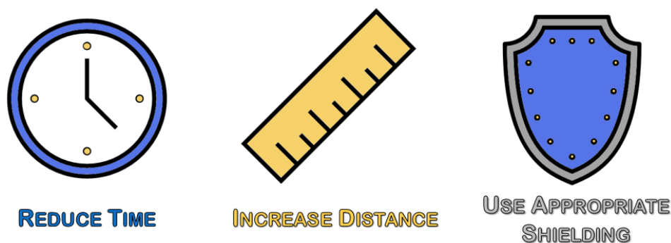
741 Fig. 3.3. The three basic rules of external radiological protection: time, distance, and shielding. 742
